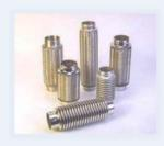
**Interlocked** metal hose assemblies are defined as a length of tubing formed from profiled strip and wound into flexible metal tubing without welding, brazing or soldering. Interlocked hose may be made pressure tight by winding in strands of packing.
